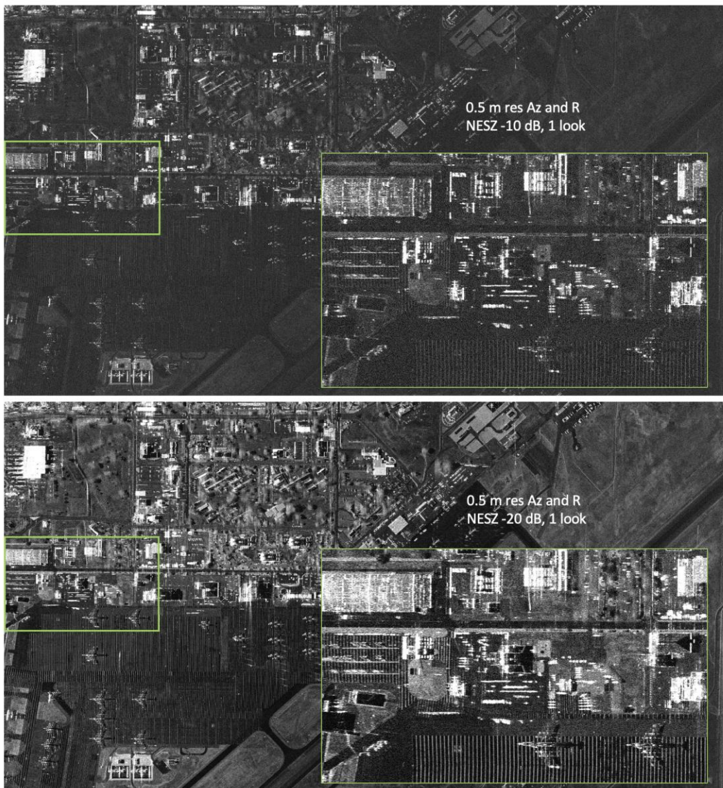
Figure 4: NESZ is a metric that informs about the system noise level in a SAR image. NESZ is usually provided as a log-scale quantity in dB, and more negative values indicate better image quality. For SAR users, the required NESZ depends on the application. Hard target detection and vegetation analysis have very different NESZ and resolution requirements.
