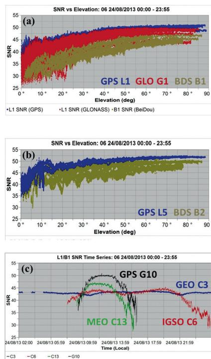
**Figure 3** Signal-to-noise ratio (SNR in dB-Hz) for GPS, GLONASS and BeiDou signal tracking (Leica Viva GS10 receiver and Leica AS10 antenna, Shanghai, open sky environment, August 24, 2013) (a) SNR vs. elevation for L1/G1/B1, (b) SNR vs. elevation for L5/B2, (c) Examples of L1/B1 SNR time series.
