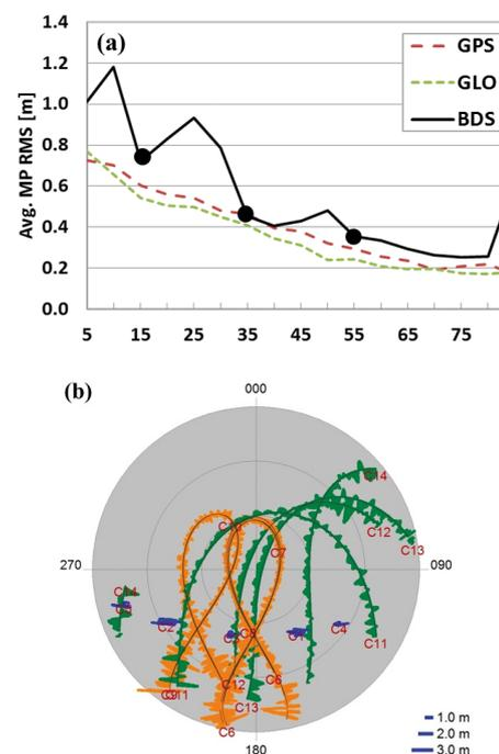
**Figure 4** Comparison of code multipath (MP) error (Shanghai, open sky environment, August 24, 2013) (a) MP vs. elevation for GPS L1, GLONASS G1 and BeiDou B1, (b) MP skyplot for the BeiDou constellation.
