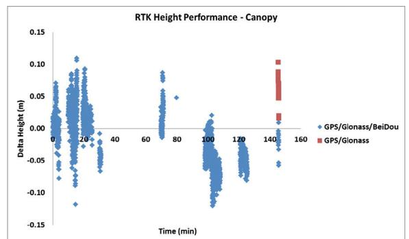
**Figure 8** RTK height errors generated using different GNSS constellations (5 km baseline RTK test in Shanghai, heavy canopy environment, August 23, 2013).
