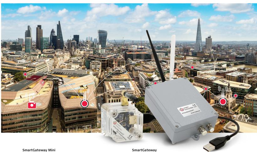
WiSenMeshWAN SmartGateway Mini is a mini USB SmartGateway for WiSenMeshWAN sensor nodes. It manages the scheduling of the connected sensors and reads data from the node and transmits it to the local data server over USB connection. Locally stored data can be pushed to the Wisen cloud or imported immediately to the monitoring software. The SmartGateway Mini is directly powered from the USB connection.
