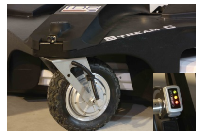
Stream C pivoting and motorized front wheel
